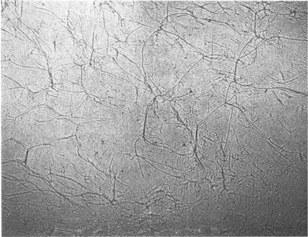
FIGURE 2. A shadowgraph of the plan view of a sugar/salt diffusive interface showing the collective instabilities.
